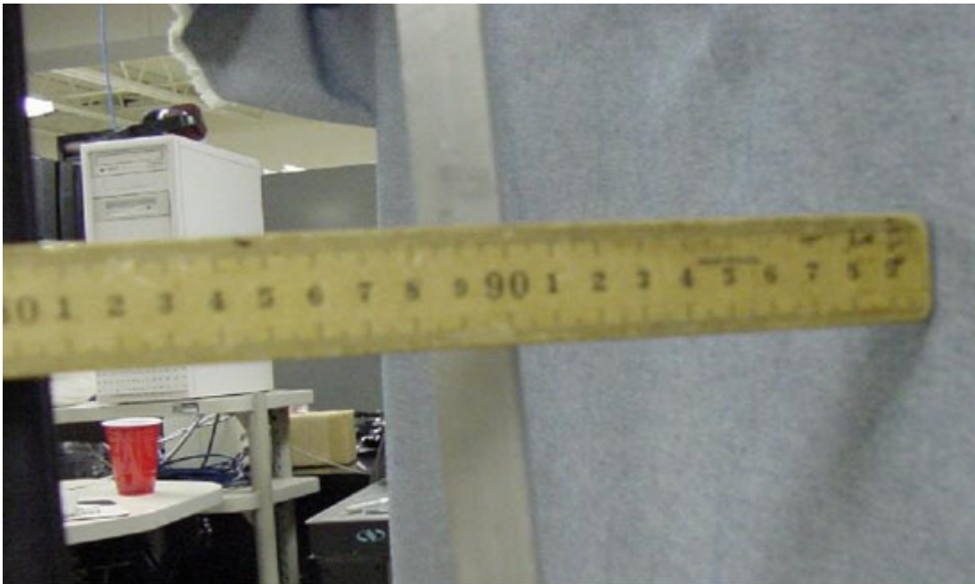
Figure 11: A photograph showing a measurement of the distance between the fabric (right) and the retroreflector (middle). From the meter stick, we see that there is a distance of 100\text{ cm} - 90\text{ cm} = 10\text{ cm} , or 0.1 meters, between the fabric and retroreflector, as was predicted from the data in Fig. 10(a).
