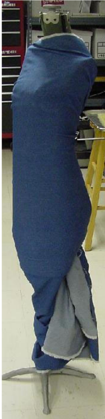
Figure 18: A photograph of No-head wrapped in a sheet of latex gum rubber and bound with denim cloth. We used this model in our first scans of No-head with rubber, but we later used ballistic gel on No-head.
