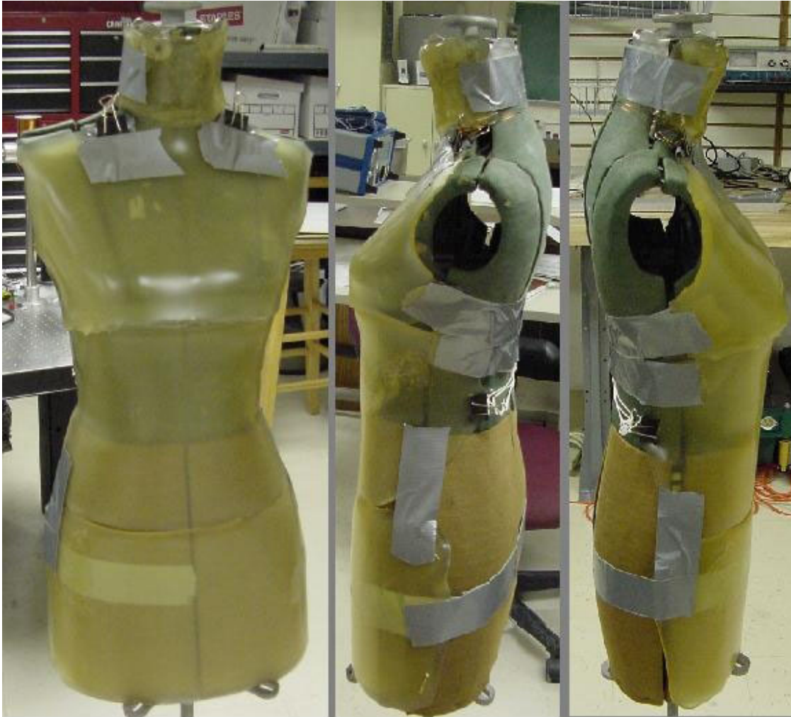
Figure 20: Three photographs of our dressmaker's dummy No-head wrapped in ballistic gel. It was constructed from three large rectangular pieces of ballistic gel melted down in an incubator and one small rectangular piece of ballistic gel for the neck.
